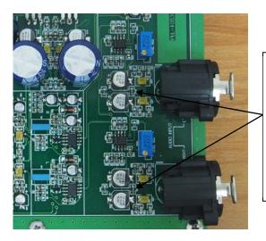
The factory set audio input impedance to 10Kohm. If you need to input impedance to 600 ohm, you will be removed SMD resistor 10kohm and replace to 600 ohm both left and right.
