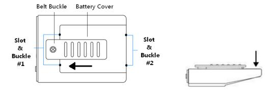
B. Uncover the buckle#2 of the battery cover, pull the cover out of the buckle#1.
